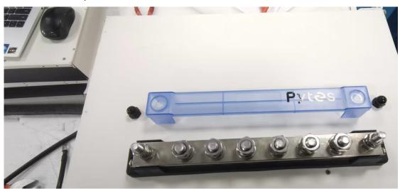
3. We can see that this busbar consists of 6 M10 terminals and 2 M8 terminals.
