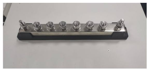
4. Remove the nut, flat washer, and spring washer from one of the M10 bolts on the busbar, align the hole of the power cable terminal with the bolt on the busbar, ensure that the power cable terminal surface is tightly attached to the busbar surface, then install the flat washer and spring washer, tighten the nut, repeat the above process, and fix the other power cables.
