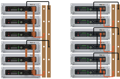
Figure 5-1 Schematic diagram of power cable connection
