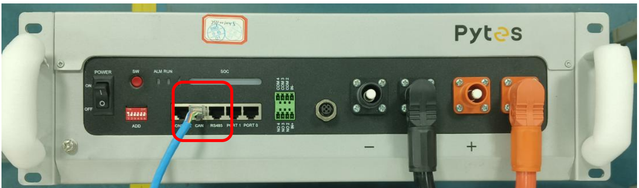
Figure 1.1.3 battery comm and power cable connection
