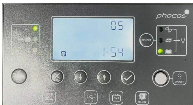
Figure 2.1.2.5 Phocos inverter battery type selection
