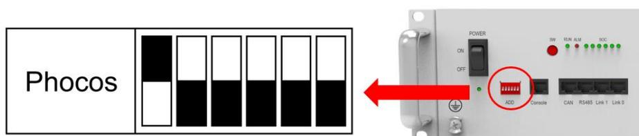
Figure 2.1.2.3 Phocos DIP switch setting
