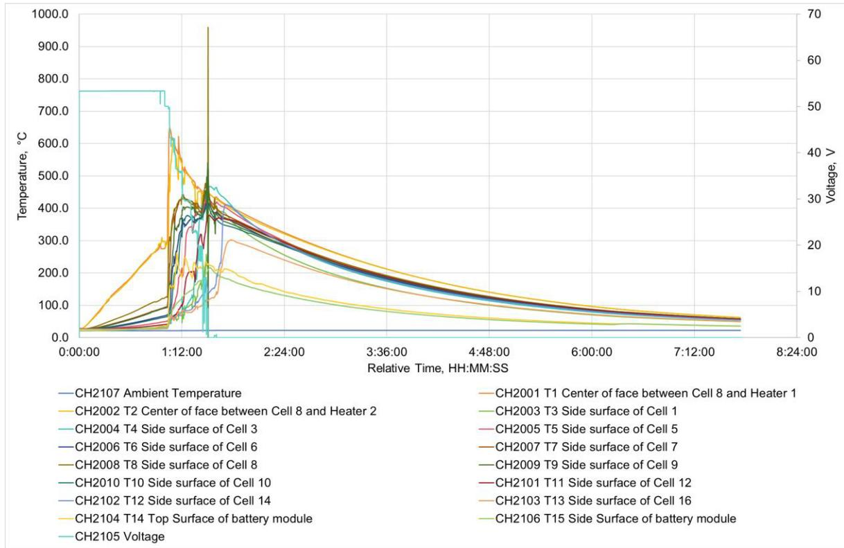
Figure 23. Temperature and Voltage measurements during test.
