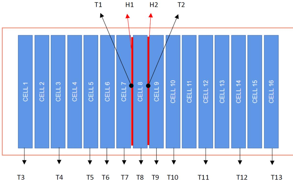
Figure 6. Schematic Illustration of film heaters and thermocouple locations in DUT (T1 to T13 means thermocouples T1 to T13. H1 and H2 means Film heater 1 and Film heater 2. View from top.).
