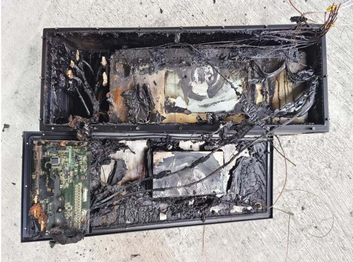
Figure 10. View of cells that exhibited thermal runaway after test.
