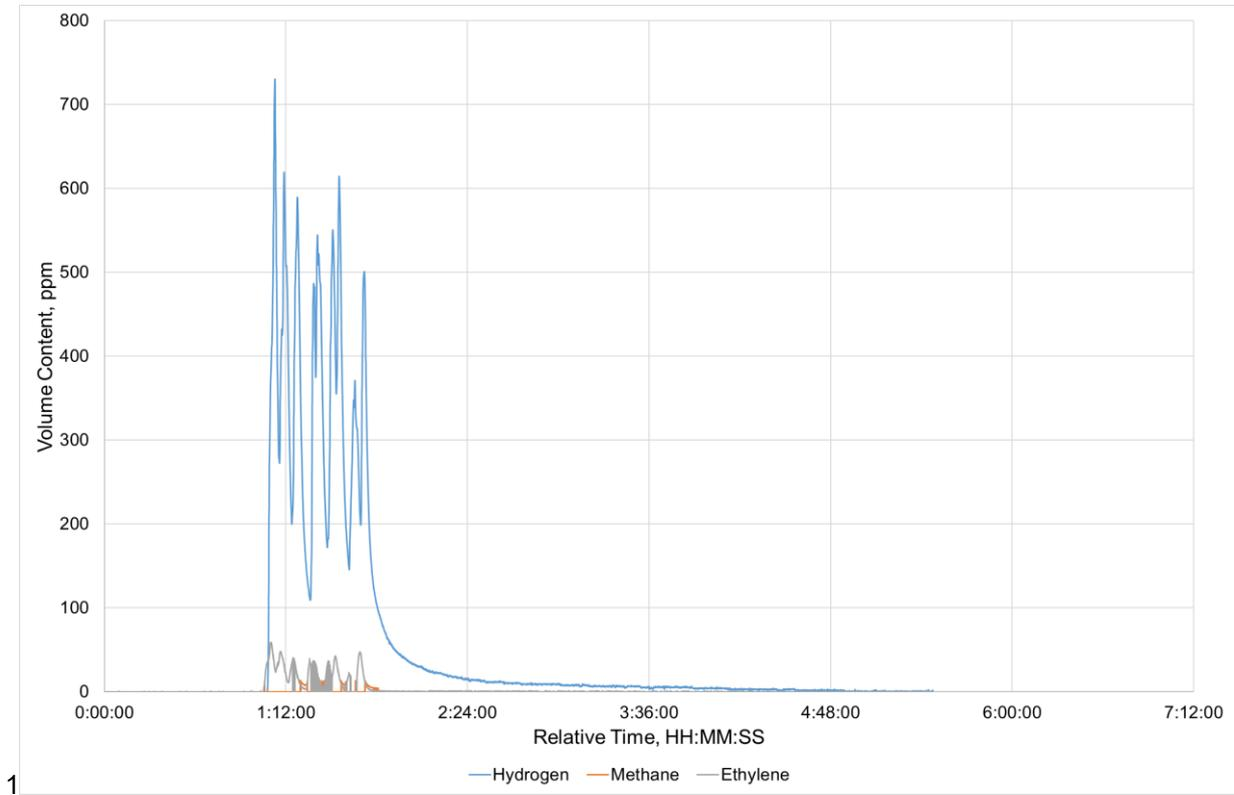
Figure 8. Online flammable gas content measurements during test. (Remark: The content of other hydrocarbons is below the detection limit of the test equipment.)
