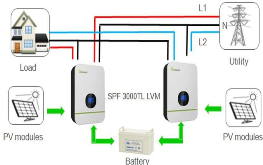
General Block Diagram of Inverter connection
