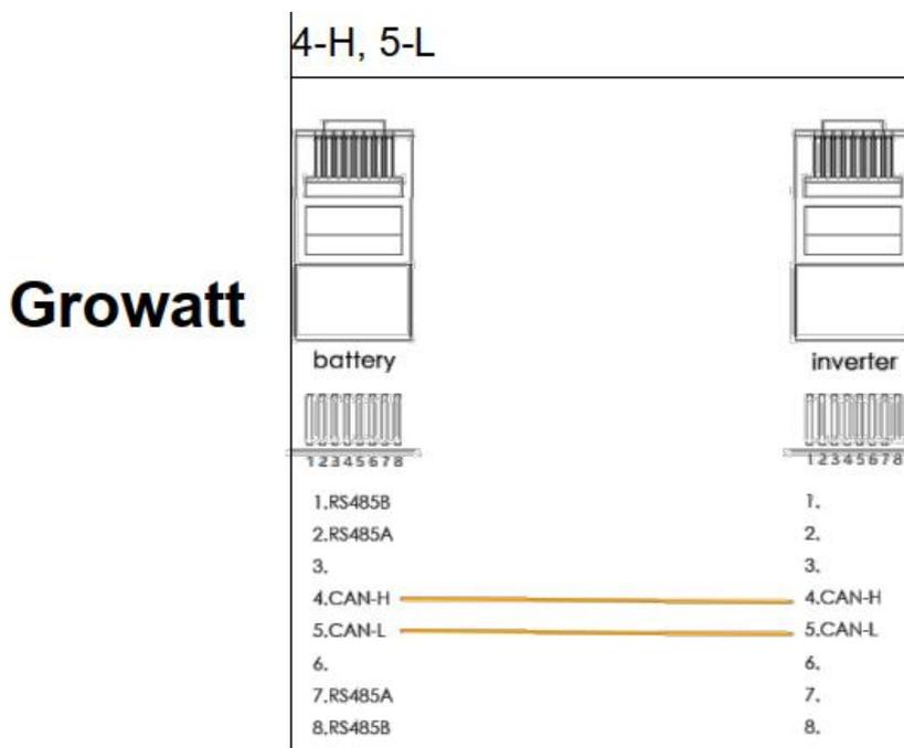
Battery and Inverter side of Communication Cable
