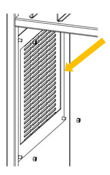
Screw the nuts and insert the filter from the gap between the mounting plate and the main body.
