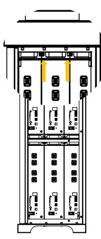
2 Fix the batteries to the main body with screws.
