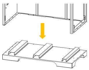
Fix the main body and the base by 10 screws.
