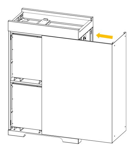
2 Fix the side cover and the main body with screws.
