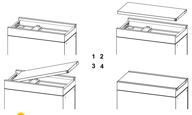
Make sure all the cables are connected, and then install the top cover as shown in the pics.
