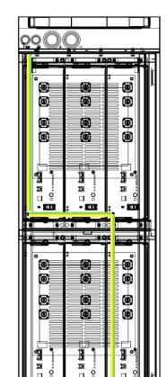
Connect the ground wire between the batteries.
