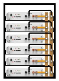
**Note**: The battery must be placed in a locked cabinet or room, and a 5cm cooling gap is reserved when installing the battery, and the battery cabinet should have a load capacity of more than 100kg
