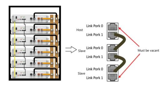
Multiple batteries: The host and the slave communicate in cascade mode: one is the host and the rest are the slaves. Please refer to the following picture for the cascade connection. User needs to insert communication cables to relevant link ports between batteries and be aware that:
